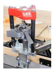
O Cycle press lever multiple times until new parts are broke-in.
