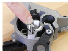
Re-insert drive bolt and driven clutch assembly and gently tap into position.
