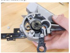
Swing clutch retainer plate back into position and tighten both Phillips screws.
