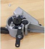
**G** Insert 3 segments into pocket of shell plate carrier
