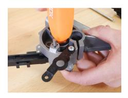
HPlace driver clutch on top of drive bolt and driven clutch assembly.
