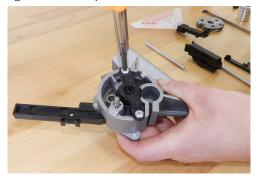
Re-install detent ball & spring, then install shell plate onto drive bolt. Verify proper installation of the 3 segments and drive bolt by making sure the shell plate freely rotates counterclockwise.
