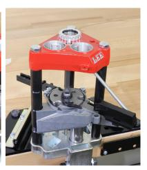
Remove case ejector and shell plate (see instructions on removing shell plate on page 7 of Pro 1000 instructions)
