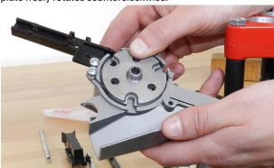
Re-install case ejector can be slid back onto the drive bolt. Place carrier on top of the ram.
