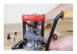
Install sizing die in station # 1. Raise ram to the top of its stroke to seat carrier in position. Tighten socket head screw 80 in./lbs. (approx. 12 ft/lbs.).
