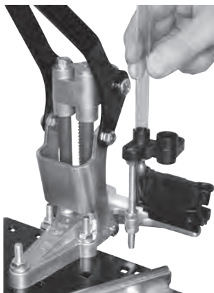
Tighten nut above rail with 7/16" wrench.
