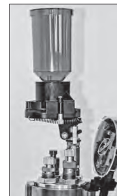
4 FLARE CASE MOUTH THIS STEP IS OMITTED WITH MOST RIFLE DIES for ease of bullet installation. Raise the ram to expand the case neck. To increase the flare, screw the die in deeper. Always adjust to provide the minimum flare needed to start the bullet. After proper adjustment, tighten the lock ring.
