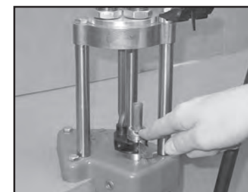
2 SIZE THE CASE Place a shell in the shell holder. Rotate the turret to position the full length sizer over the case. Firmly raise the ram to the top and stop.
