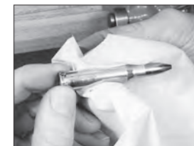
6 IF LOADING maximum loads, it's good practice to remove all traces of case lubricant with detergent and water. This reduces pressure against the bolt.
