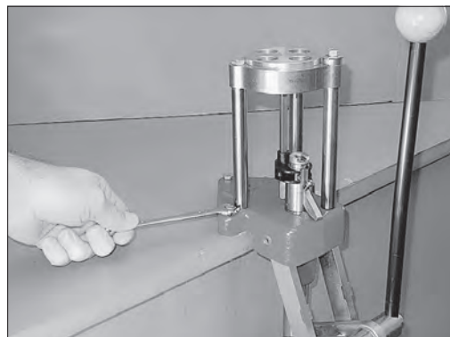
FIGURE 1 Attach the Classic Turret Press to the front edge of a sturdy bench using three 1/4 or 5/16 inch bolts.
