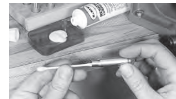
RIFLE DIES ONLY Be sure to lube the inside of the case neck with a cotton swab.
