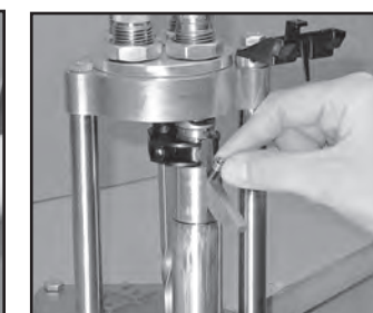
3 SELECT CORRECT LEVER PRIME ASSEMBLY (large or small). With clean fingers, place the correct size and type of primer in the primer guide. (This operation is greatly speeded by using the Lee Safety Prime primer feeder. Never touch the primer from box to shell.) Seat the primer by lowering the ram—lifting up on the press lever. Lift firmly enough to seat the primer flush to slightly below flush of the case head.
