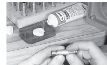
Carbide dies need no lubrication
