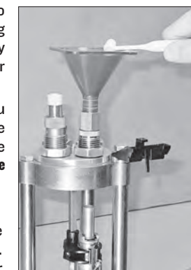
4 FLARE CASE MOUTH THIS STEP IS OMITTED WITH MOST RIFLE DIES for ease of bullet installation. Raise the ram to expand the case neck. To increase the flare, screw the die in deeper. Always adjust to provide the minimum flare needed to start the bullet. After proper adjustment, tighten the lock ring.
