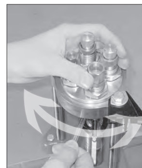
4 FLARE CASE MOUTH THIS STEP IS OMITTED WITH MOST RIFLE DIES for ease of bullet installation. Raise the ram to expand the case neck. To increase the flare, screw the die in deeper. Always adjust to provide the minimum flare needed to start the bullet. After proper adjustment, tighten the lock ring.
