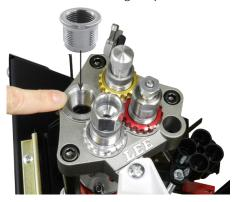
Install action rod into feeder link. Use end hole as shown.
