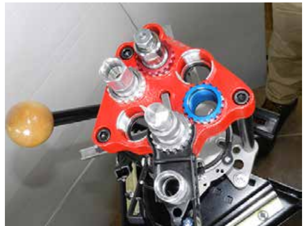
Install bullet seating die with lock ring on and feeder assembly into position 4. Verify the action rod is close to vertical.
