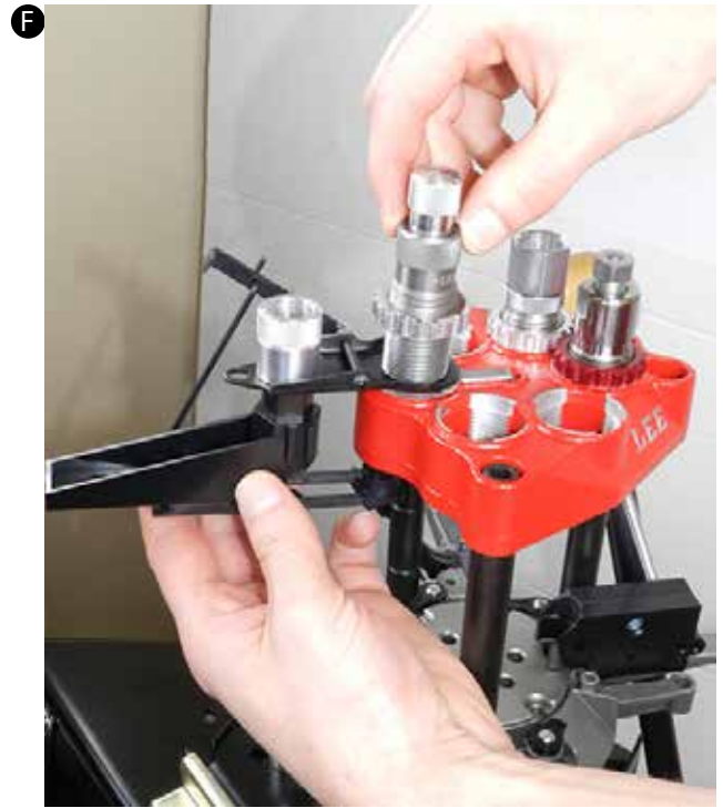
Install bullet seating die with lock ring on and feeder assembly into position 4. Verify the action rod is close to vertical.
