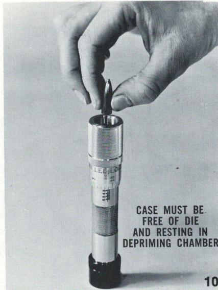
**CASE MUST BE FREE OF DIE AND RESTING IN DEPRIMING CHAMBER.**
