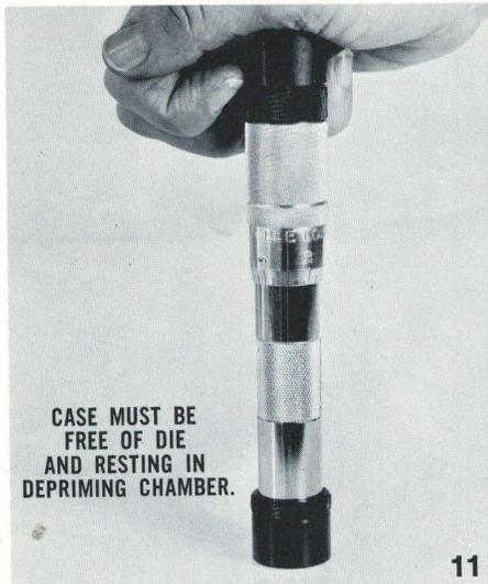
**CASE MUST BE FREE OF DIE AND RESTING IN DEPRIMING CHAMBER.**
