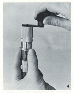
With the micrometer set at zero ream the neck of the case. IM-PORTANT: See "NECK REAMING" in this instruction sheet. CASES MUST BE FIRED FROM YOUR GUN. DO NOT REAM NEW UNFIRED CASES.
