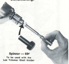
Speed up your case preparation with this handy tool. The  $\frac{1}{4}$ " shank fits any hole shooter or drill press. All the operations can be done without removing the shell or stopping the motor.
