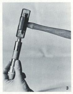
Drive the case into the Loader until the head is flush. A plastic mallet works best but a piece of hardwood 10 or 12 inches long works well.
