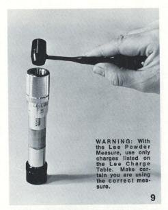
Place the case in the head alignment chamber and slip the body die assembly over the case. Add a charge of powder. Refer to the charge table for the proper load.
