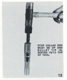
Crimp the bullet only on tubular magazine guns. Place the cartridge in the loading tool as pictured (Fig. 12) with bullet down and the depriming chamber on the head. Tap lightly until the desired crimp is formed. This can only be done with bullets having a crimping groove, or lead bullets.
