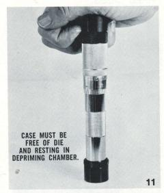
Insert the bullet seater and push down until it stops against the stop collar. It may be desirable to use a light mallet for the first loading of once fired cases.
