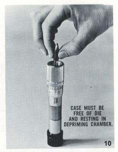
Drop a bullet into the top of the tool. The bullet depth adjustment should have been previously set. (SEE MICROMETER BULLET DEPTH ADJUSTMENT.) Set stop to any desired bullet depth. It is necessary to readjust to zero whenever bullet shape or weight is changed.
