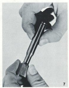
Chamfer the inside and outside of the case. Use only one turn with light pressure. DO THIS ONLY THE FIRST TIME OR AFTER CASE TRIMMING.
